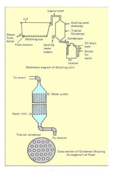
to produce steam, a distillation tub, a condenser and one to three separators. The distillation tub
